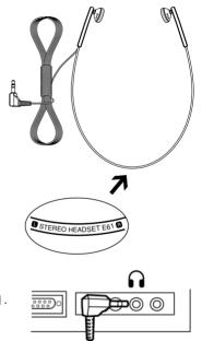
Plug the headset into the PC's earphone terminal .
