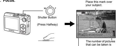
When the focus and exposure are locked, the green lamp lights up, and the shutter speed and aperture value are displayed.
