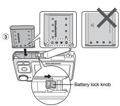
Insert the battery by putting in the ▼ marked side first, with the ➡ marks toward the battery lock knob.
