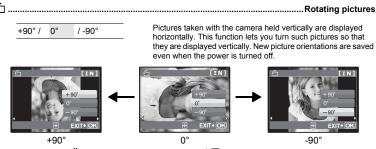
Select a picture with  $\triangle$ , and select [+90°]/[0°]/[-90°] with  $\triangle$  to rotate pictures. You can rotate several frames in succession.
