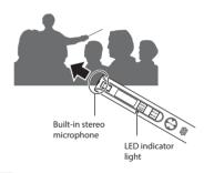
Slide the REC switch to start recording in the direction of the arrow.
