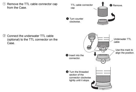
How to attach the TTL cable connector cap to the case
