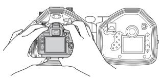
(5) When using an external electronic flash with a TTL cable, connect the hot shoe cable to the camera's hot shoe and set the camera's automatic pop-up setting to OFF.
