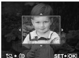
**[ASPECT]** Changes the aspect ratio of images from 4:3 (standard) to **[3:2]**, **[16:9]**, or **[6:6]**. After changing the aspect ratio, use the arrow pad to specify the trimming position.
