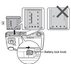
Insert the battery by putting in the ▼ marked side first, with the ♠ marks toward the battery lock knob.
