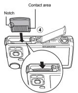
Orient the card as shown in the illustration and insert it straight into the card slot.
