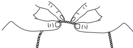
Use a clean cloth not easily shedding fibers or a toothbrush or tissue paper or the like to remove any foreign matter from the O-ring groove. Clean the O-ring contact surface on the front lid in the same way to remove any sand and dirt.
