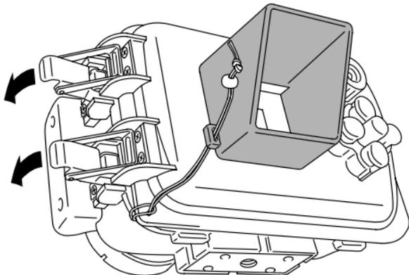
**CAUTION** : • Seal the Case by turning both buckle lock levers down in arrow direction. When one of the buckles is left open, the Case will not be sealed and water leakage will be caused.
