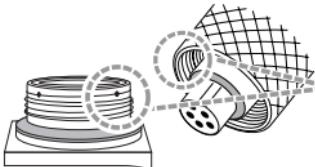
Clean and apply O-ring silicon grease to these sections.
