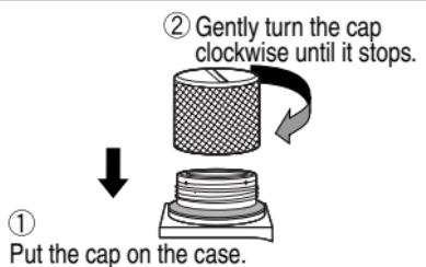
**CAUTION:** • If the TTL cable connector cap is loose, water penetration may result. Be sure to gently turn the cap until it stops to make sure it is firmly secured. Do not turn or tighten the TTL cable too hard. If it is too tight, it may be difficult to loosen and remove it.
