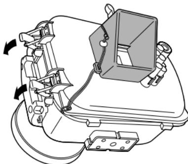
**CAUTION:** • Seal the Case by turning both buckle lock levers down in arrow direction. When one of the buckles is left open, the Case will not be sealed and water leakage will be caused.
