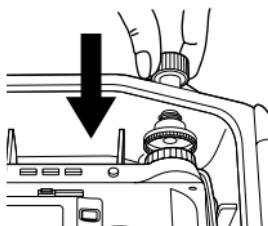
**Advice** • After setting the mode dial of the case, set the power of the digital camera to 'OFF', and before sealing the case, operate the mode dial and confirm that the mode of the digital camera is switched.
