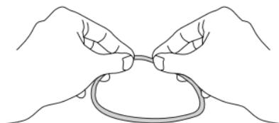
Remove any foreign matter adhered to the O-ring groove using a lint-free clean cloth or cotton swab. Also remove any sand or dirt adhered to the O-ring contact surfaces on the front and rear lids of the Case.
