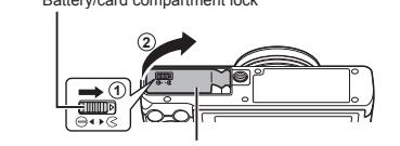
**2** Insert the battery while sliding the battery lock knob in the direction of the arrow.
