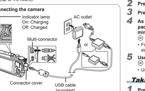
**2** Never use any cable other than supplied or Olympus-designed USB cable. This may cause smoking or burning.
