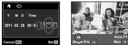
Operation guides displayed at the bottom of the screen indicate that the **MENU** button,  $\odot$  button, or zoom lever can be used.
