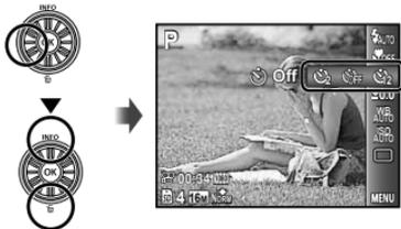
**2** Use  $\triangleleft$  and  $\triangleright$  to select the setting option, and press the  $\odot$  button to set.
