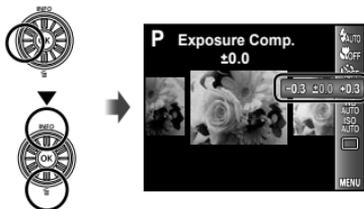
**2** Use  $\triangleleft$  and  $\triangleright$  to select the desired brightness, and press the  $\odot$  button.
