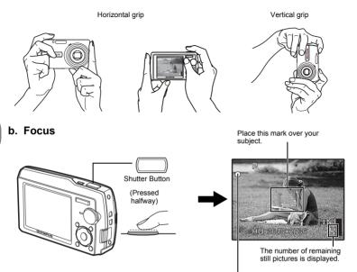
The green lamp indicates the focus and exposure are locked.
