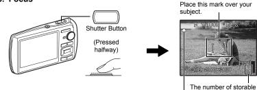
When the focus and exposure are locked, the green lamp lights up, and the shutter speed and aperture value are displayed.
