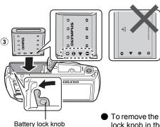
To remove the battery, slide the battery lock knob in the direction of the arrow.
