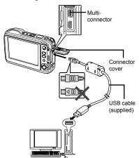
When [USB Connection] is set to [Auto], connect the camera and the computer, select [Storage] or [MTP] at the screen for selecting the connection method, and then press the (a) button.
