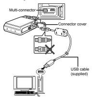
When [USB Connection] is set to [Auto], connect the camera and the computer, select [Storage] or [MTP] at the screen for selecting the connection method, and then press the (@) button.
