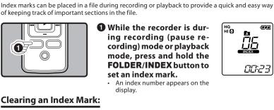
**1** While the recorder is during recording (pause recording) mode or playback mode, press and hold the FOLDER/INDEX button to set an index mark. An index number appears on the
