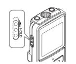
Power on: Slide the HOLD switch in the direction opposite that indicated by the arrow. Power off: Slide the HOLD switch in the
