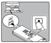
When charging the battery, press and hold the STOP (■) button until [Please Wait] is displayed.
