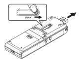
3 After making sure the voice recorder is in stop mode, connect its USB connector to a USB port on the PC.
