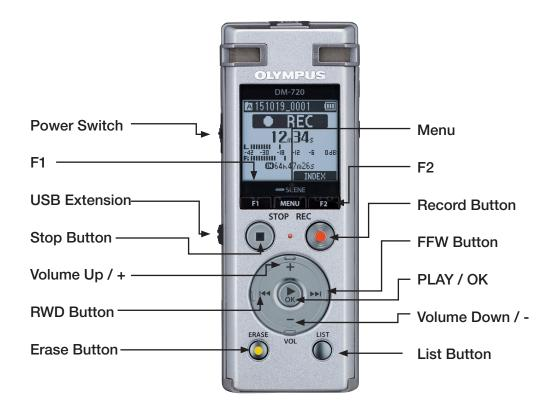
To turn on the DM-720 slide the Power button located on the side to power position and release.
