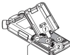
Insert batteries' negative terminals first.
