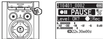
**5** Press the **▶▶** or **◀◀** button to adjust the recording level.
